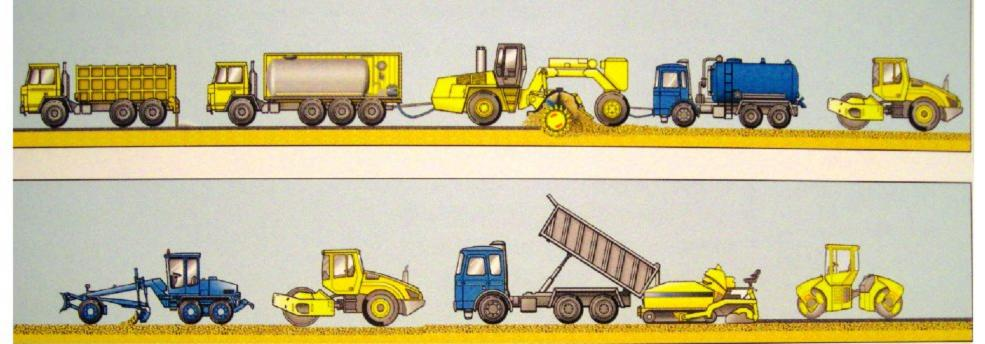
The road recycler is efficient, economical and environmental road construction equipment, produced by our company for the urban and rural road rebuild. In recycling work, it can mill, pulverize old asphalt road, and mix together with stablizer, cement (or lime) and water (or emulsified asphalt) into the new road base. The machine also is used for stabilization in place of soil material with lime, cement, or asphalt in road construction.
